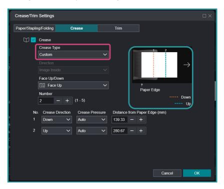
4. You can adjust either face up or face down under Face Up/Down options. Number of creases can be adjusted under the Number option. Other settings such as direction, pressure, and distance can also be adjusted following Crease Direction, Crease Pressure, and Distance from Paper Edge (mm) options.
