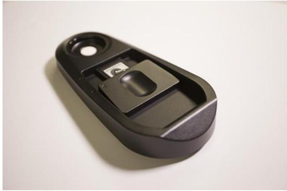
**Figure 7:** i1Pro 2 Spectrophotometer “White reference plate”
