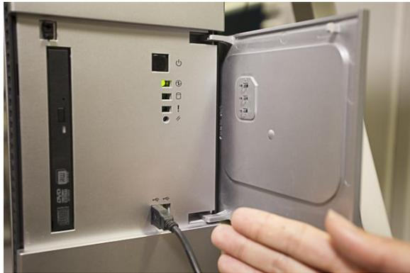
**Figure 1:** Connect USB port on the front of the GX Print Server
