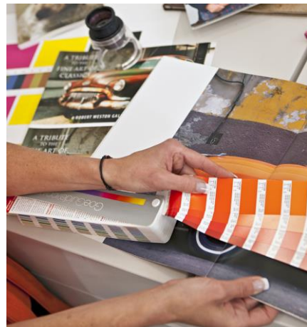
Colour matching using CMYK standards
