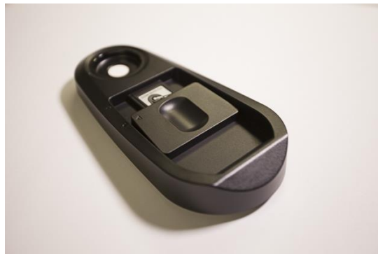
Figure 4: i1Pro 2 Spectrophotometer "White reference plate".
