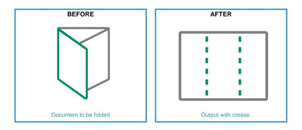
A physical Crease can be applied when the optional Crease/Two-sided Trimmer is installed on the printer.
