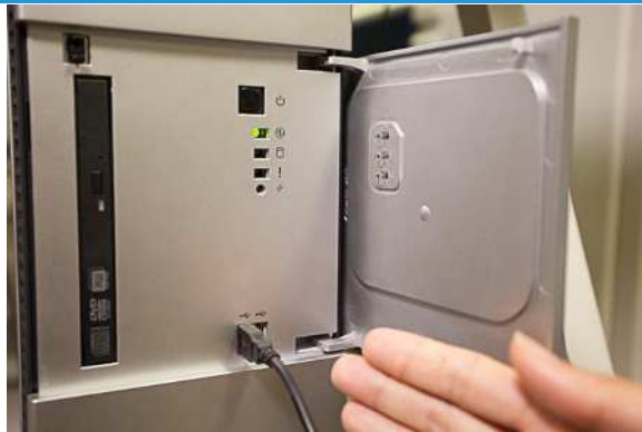
Figure 2: Connect USB port on the front of the GX Print Server.
