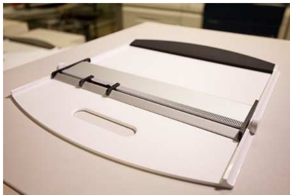
Figure 1: Calibration “Backup Board” used for A4 paper.
