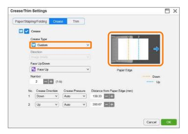
3. You can adjust either face up or face down within the [Face Up/Down] option. As well as the number of creases using the [Number] option. You can also configure the direction of the crease using [Crease Direction], the pressure of the crease using [Crease Pressure], and the position of the crease using [Distance from Paper Edge (mm)] for each crease.
